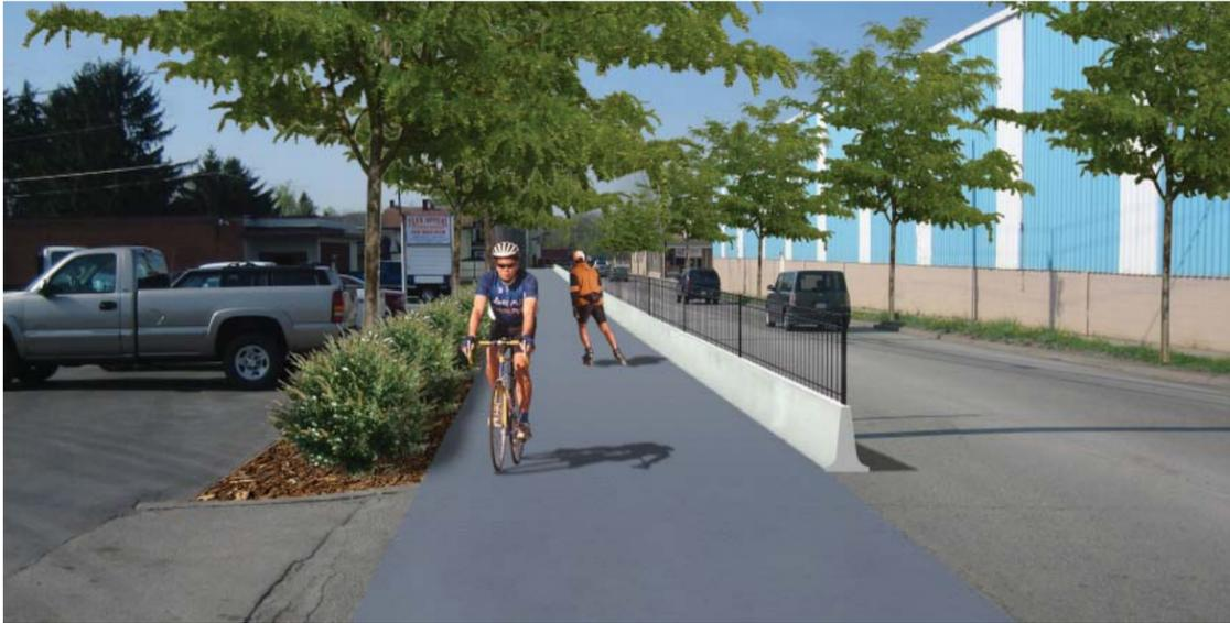
Buffer segregates motor vehicle traffic from bike lane, mixed-use trail or sidewalk.
