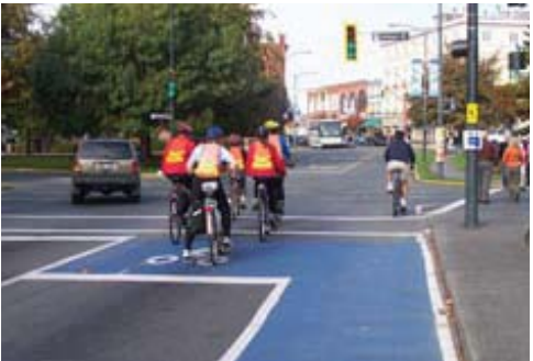
Above and below: Bike boxes filled in with color to emphasize allocation of space to bicycle traffic.
