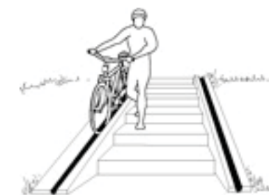
Bicycle wheel gutters on stairs and boardwalk bridge
