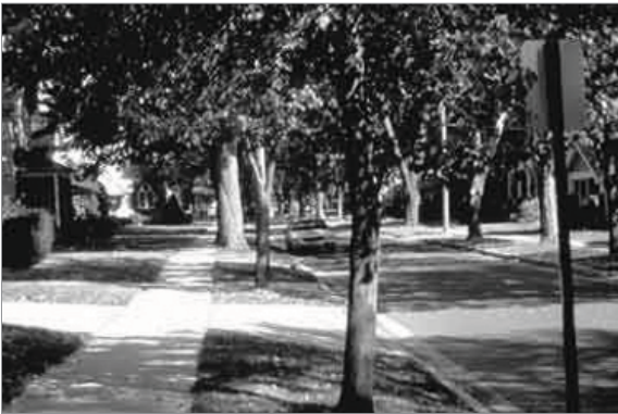
A well designed residential sidewalk will have a width of at least five feet. (Image from http://www.walkinginfo.org )
